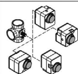
Installation position of the fixed setpoint controller. The display always adapts to the installation position of the fixed setpoint controller on the mixer.
