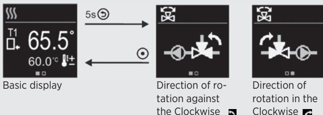
The setting can be adjusted with the  $\oplus$  and  $\ominus$  keys and confirmed with the key  $\odot$
