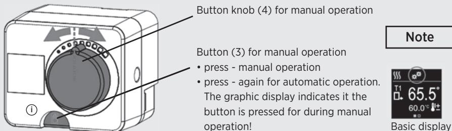
**6 Assembly of fixed setpoint controller SM WR FR**
