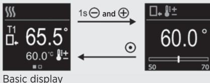
The setting can be adjusted with the buttons  $\oplus$  and  $\ominus$  in  $1^\circ$  steps and confirmed with the  $\odot$  button. The change is immediately shown on the display and the fixed setpoint controller operates under the new setting.
