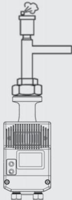
Fill system properly and vent. To vent the pump, this should be done as in chapter 7.3 Section IV. After this process, the pump can be set in the desired control mode.
